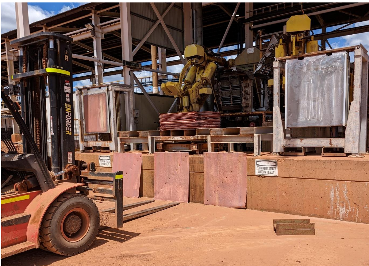
Figure 5. Copper stripping machine with sample sheets. Samples being sent for assaying
