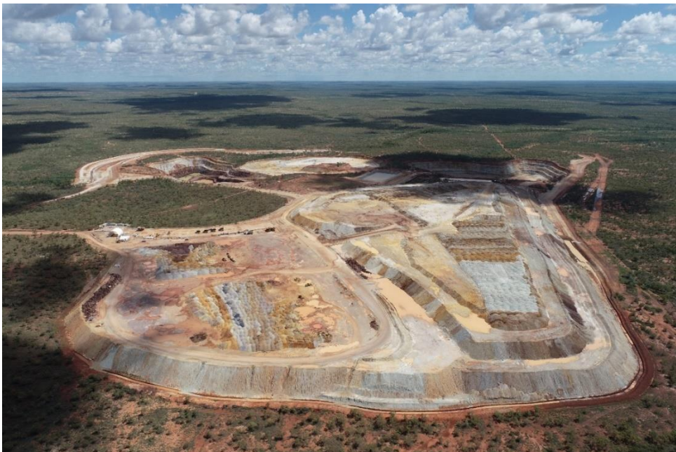
Figure 2. View of the Anthill mine with the ROM pad and waste dump in the foreground
