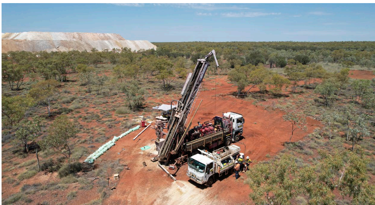
Figure 4. Exploration drilling to north west of Anthill mine, waste rock dumps in background
