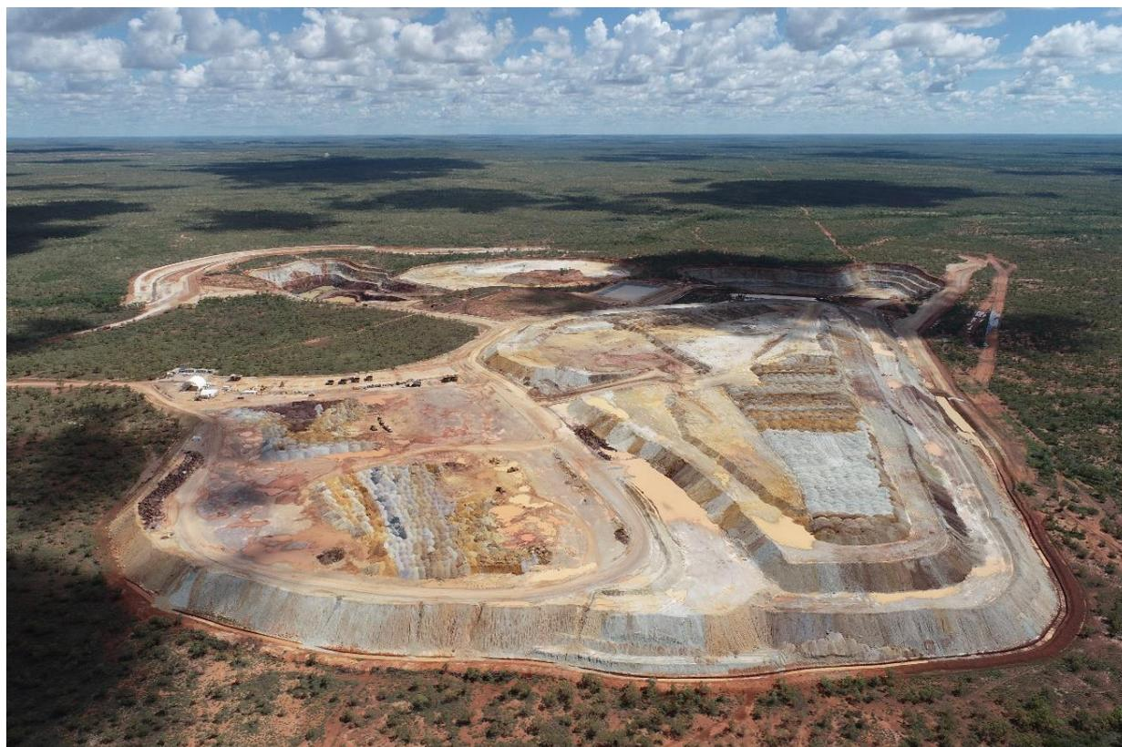
Figure 4 View of the Anthill mine with the ROM pad and waste dump in the foreground
