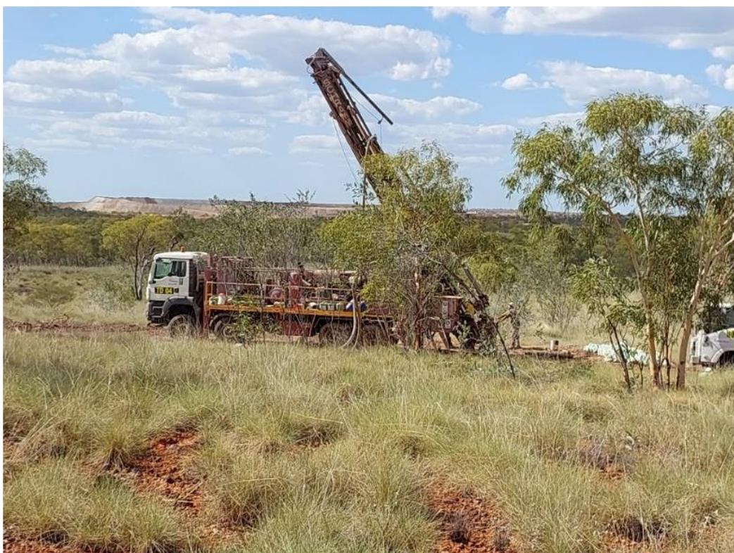
Figure 6 Tulla RC rig TD04 drilling Anthill 2.0 BURC00686, Anthill waste dumps in background
