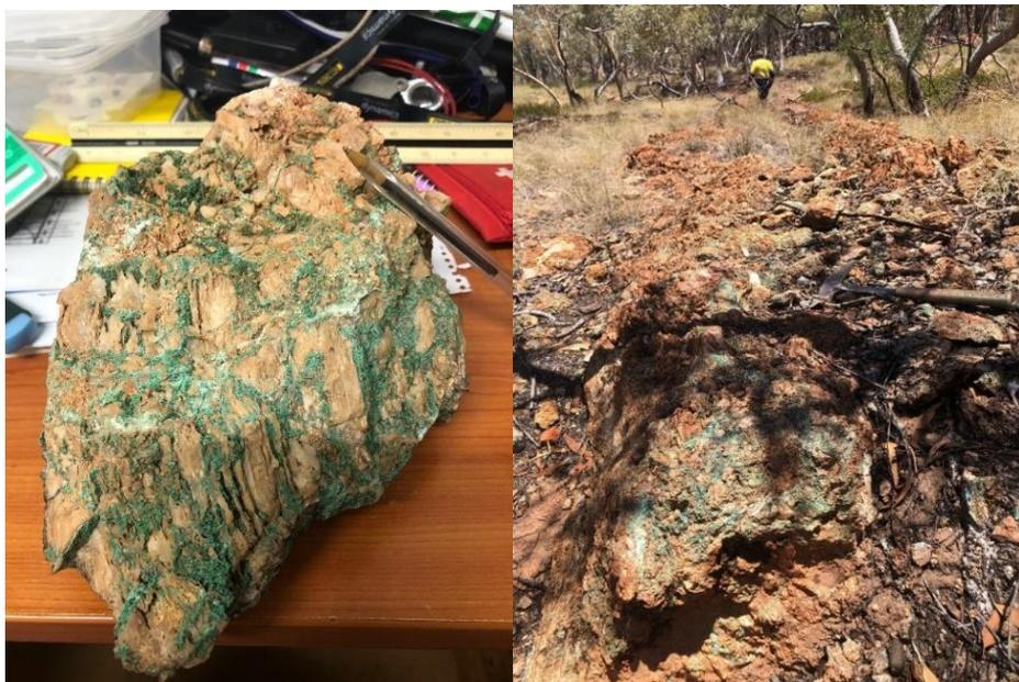
*Figure 8 Busy Bee copper oxide mineralisation (16.05% Cu) looking south and Malachite infill in quartz fault breccia*
