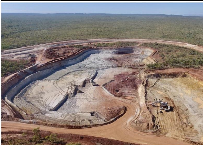
Figure 2: Anthill Mine east pit – oxide Cu ore on RHS of main pit as dark coloured material
