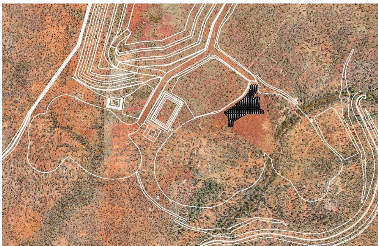
Figure 4. Anthill pit shells showing cleared areas to date and first blast footprint at the east pit, shaded black.
