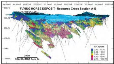
Figure B12: Cross section of the Flying Horse deposit showing drilling, copper grade ranges of resource model blocks and open pit
