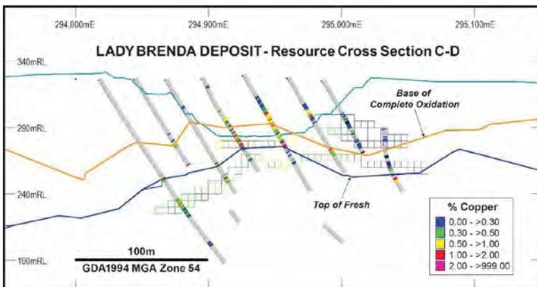
Figure B7: Cross section C-D of the Lady Brenda deposit showing drillholes and copper grade ranges of resource model blocks (base of open pit in blue)
