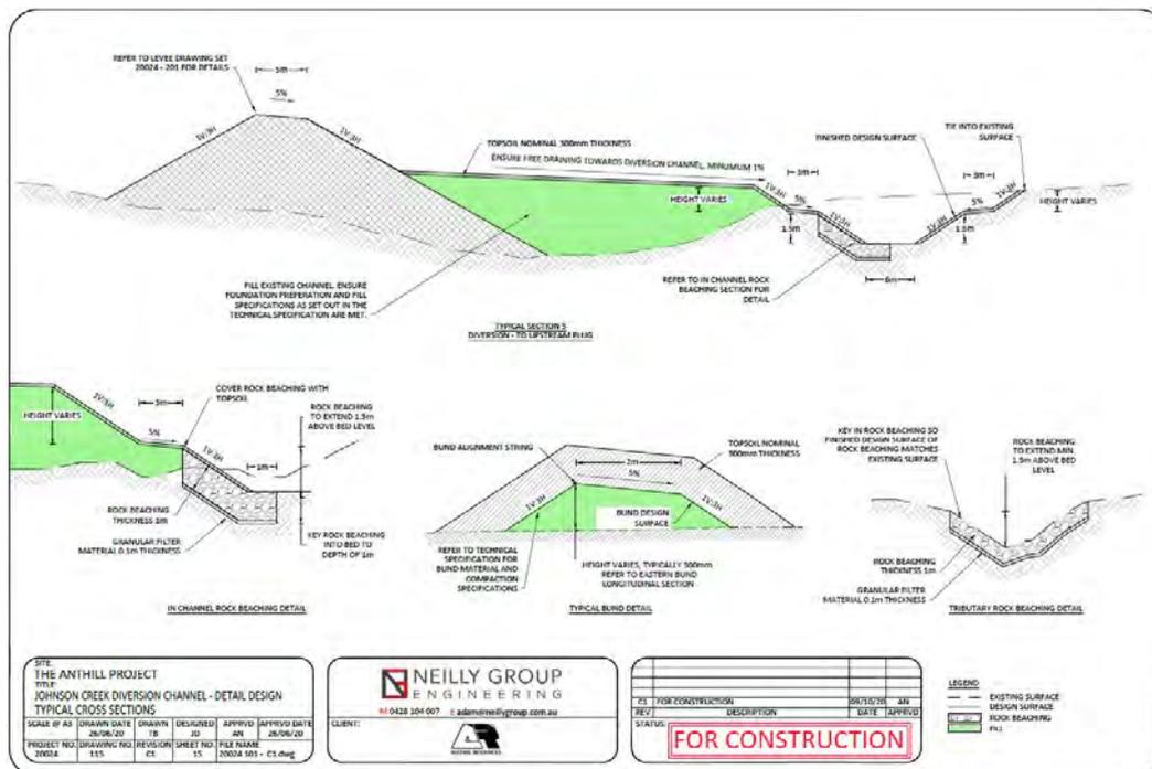
Figure 14: Neilly Group Engineering (2020) typical design sections for upstream plug, in channel rock beaching detail, bund detail, tributary rock beaching detail
