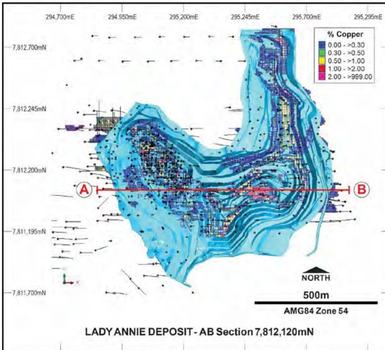
Figure B1: Plan of the Lady Annie deposit showing drilling, pit outline and block model coloured by copper grade
