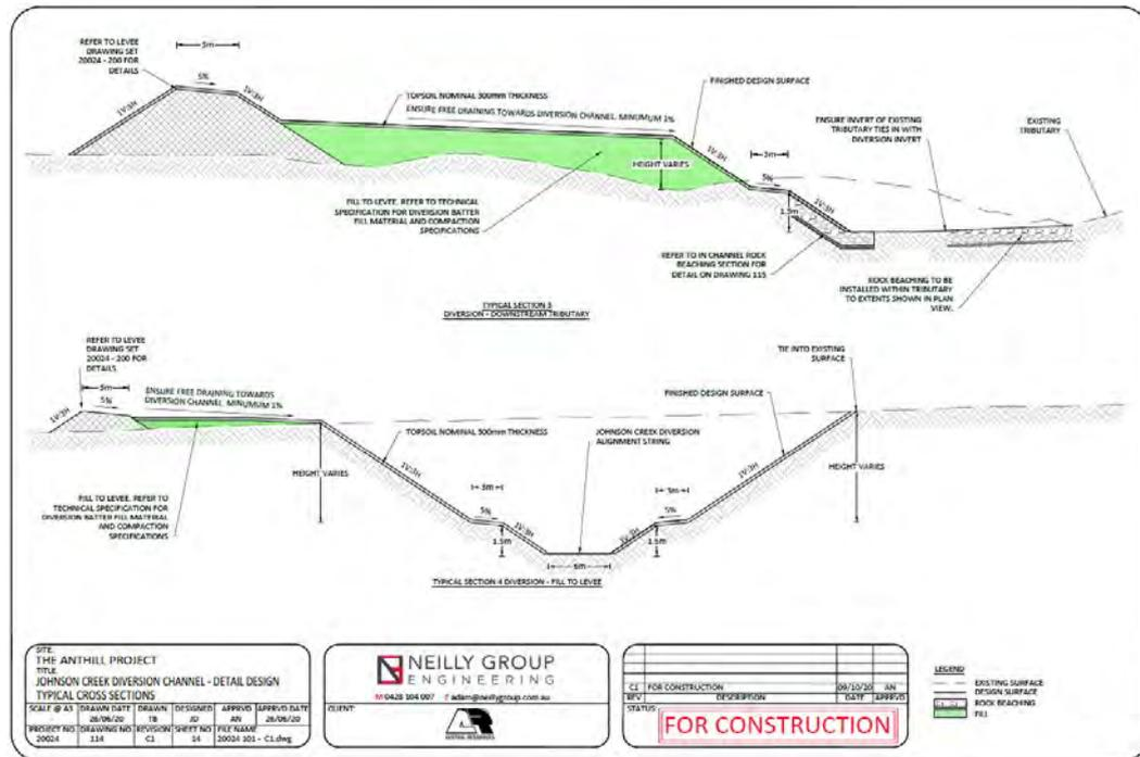
Figure 13: Neilly Group Engineering (2020) typical design sections for downstream tributary and fill to levee
