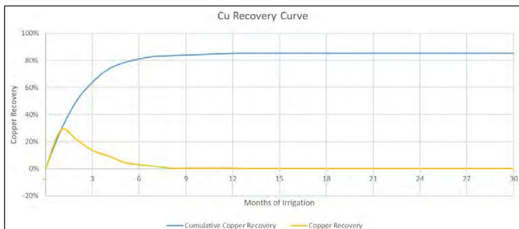
Figure 1: Copper recovery curve
