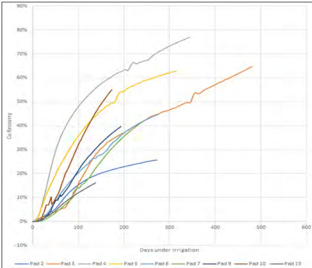
Figure 24: Copper recovery vs days under irrigation, pads 2 to 13 from the remnant mining campaign
