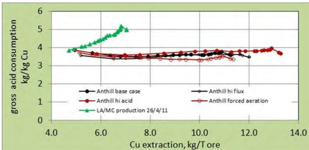
Figure 22: Increased acid concentration vs copper extraction
