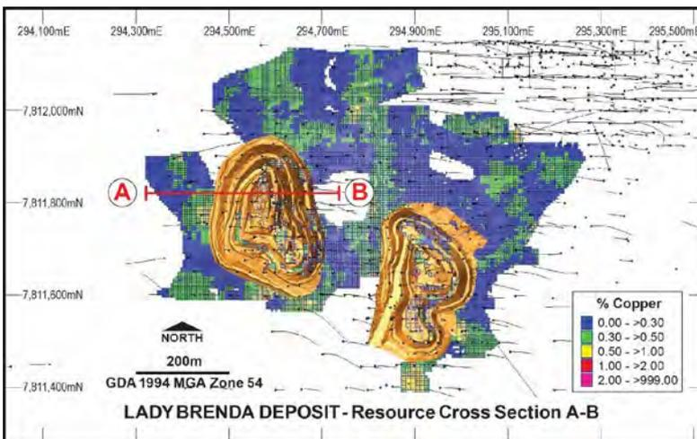
Figure B5: Plan of the Lady Brenda deposit showing drilling, pit outlines and block model coloured by copper grade
