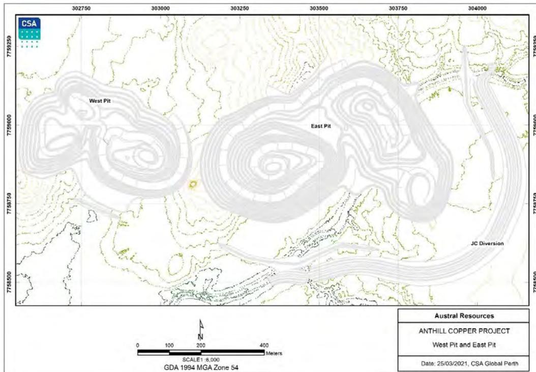
Figure 11: Final (stage 4) pit design with Johnson Creek diversion channel
