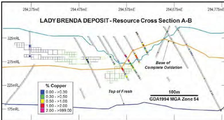
Figure B6: Cross section A-B of the Lady Brenda deposit showing drillholes and copper grade ranges of resource model blocks (base of open pit in blue)
