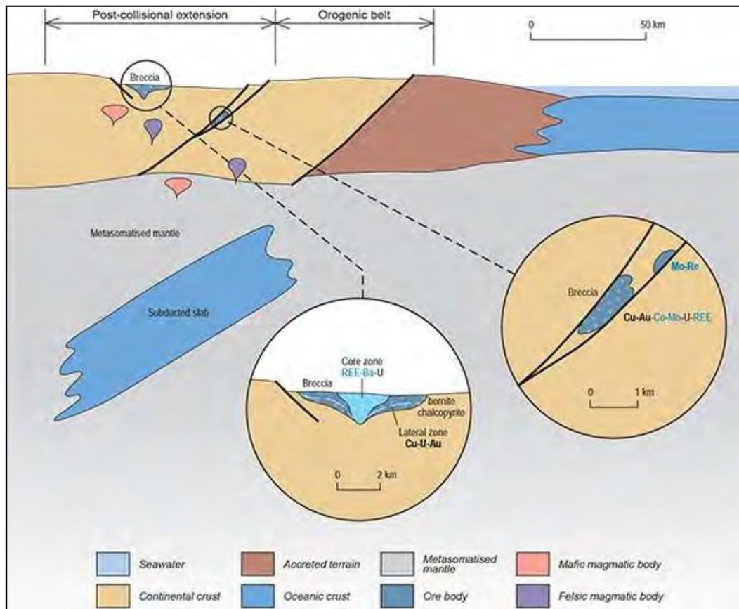
Figure 28: Geological model of an IOCG mineral system
