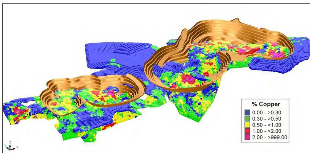
Figure 7: Isometric view of the Anthill deposit showing the resource block model and planned open pit
