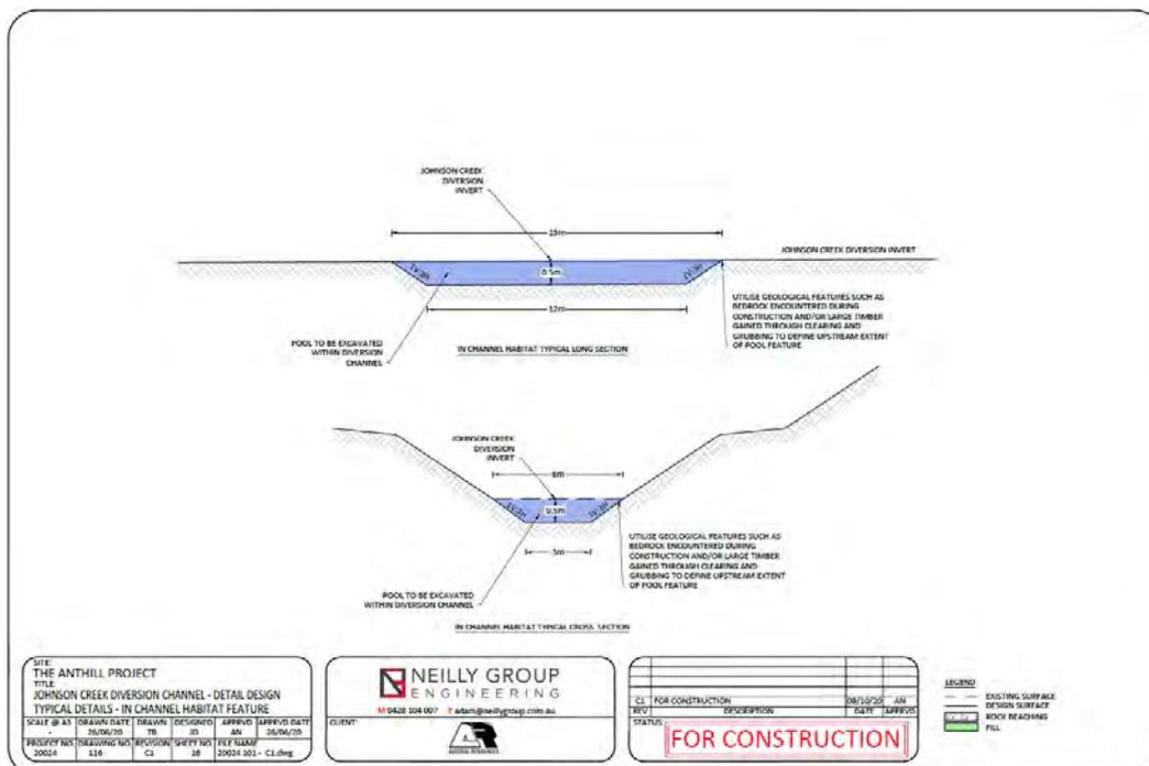
Figure 15: Neilly Group Engineering (2020) typical design sections for in channel habitat
