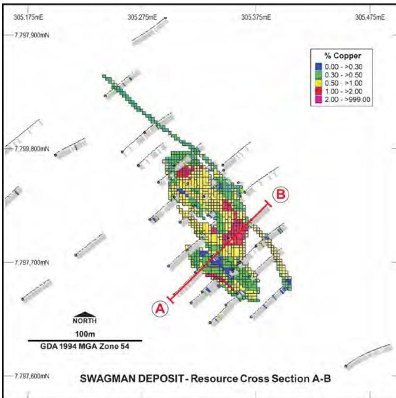
Figure B14: Plan of the Swagman deposit showing drillholes and copper grade ranges of resource model blocks
