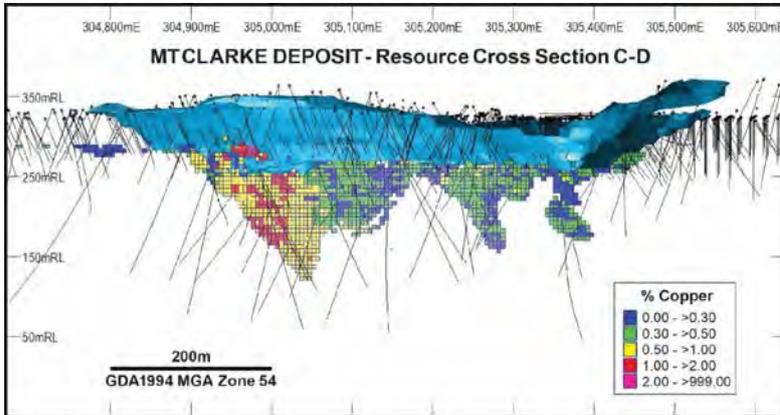
Figure B13: Cross section of the Mount Clarke deposit showing drilling, copper grade ranges of resource model blocks and open pit
