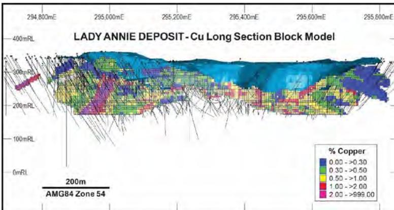
Figure B4: Long section of the Lady Annie deposit showing copper grade ranges of resource model blocks, drillholes and open pit
