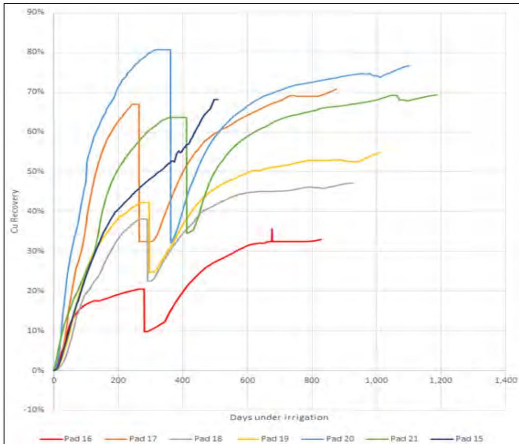
Figure 25: Copper recovery vs days under irrigation, pads 15 to 21 from low-grade stockpiles
