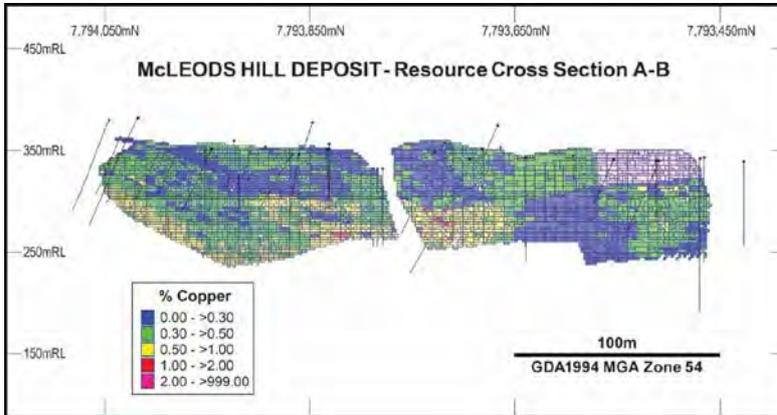
Figure B17: Cross section of the McLead Hill deposit showing drilling and copper grade ranges of resource model blocks
