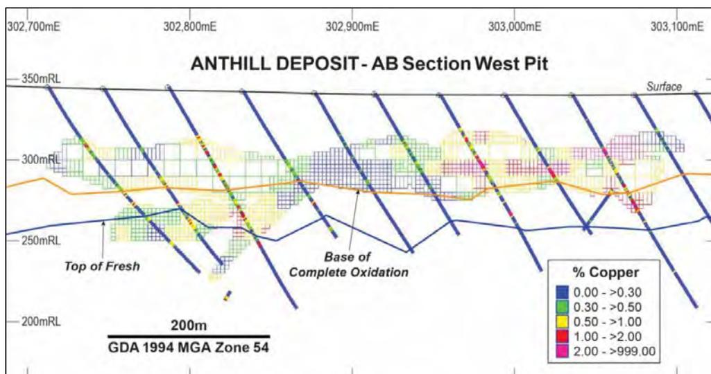
Figure 8: Cross section of the Anthill deposit showing drillholes and block model coloured by copper grade
