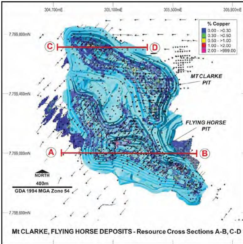
Figure B11: Plan of the Flying Horse deposit showing drilling, interpreted mineralisation as resource model blocks and existing open pit
