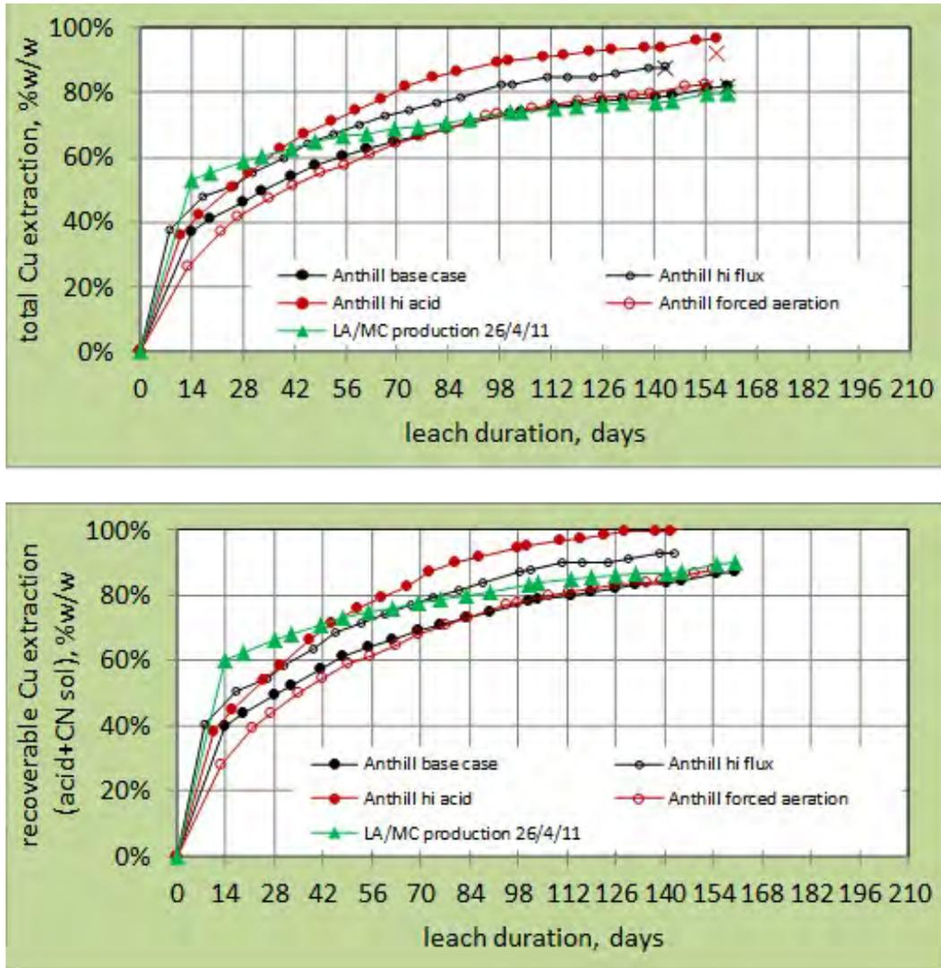
Figure 21: Copper leach extraction vs time
