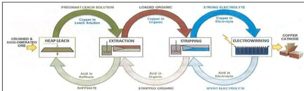
Figure 23: Heap leach and SX-EW flowsheet
