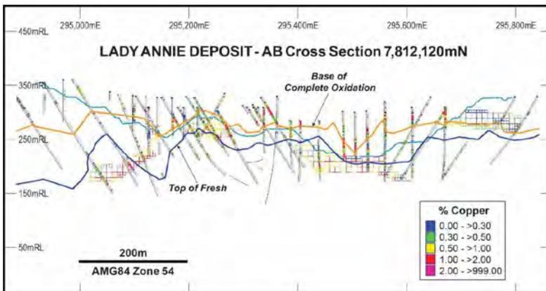
Figure B2: Cross section A-B of the Lady Annie deposit showing drillholes and block model coloured by copper grade (base of open pit in blue)
