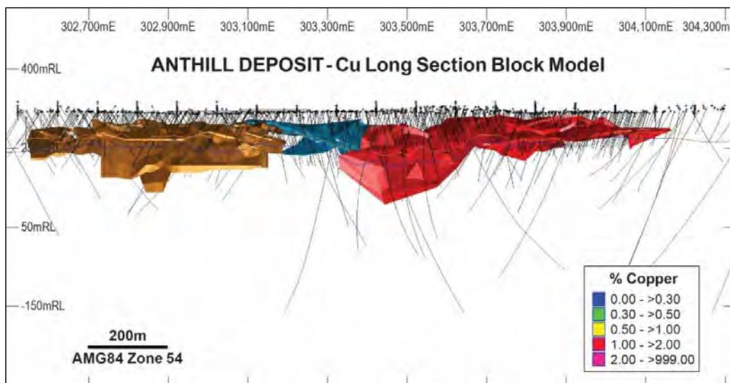
Figure 9: Long section of the Anthill deposit showing all drillholes and interpreted mineralisation wireframes
