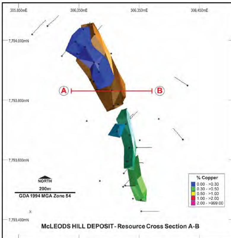
Figure B16: Plan of the McLeod Hill deposit showing drilling, interpreted mineralisation and
