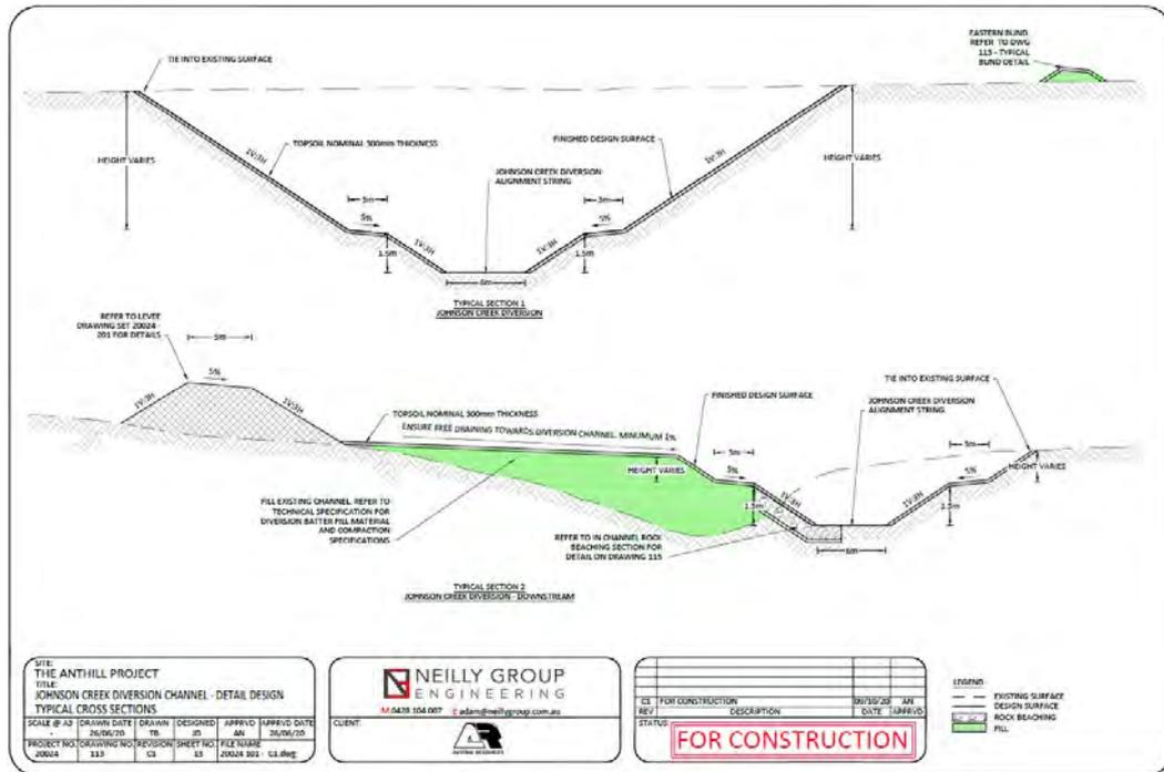
Figure 12: Neilly Group Engineering (2020) typical Johnson Creek diversion design sections 1 and 2
