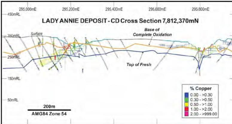
Figure B3: Cross section C-D of the Lady Annie deposit showing drillholes and block model coloured by copper grade (base of open pit in blue)
