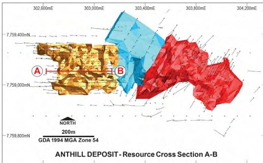
Figure 6: Plan of the Anthill deposit showing drilling and interpreted mineralisation wireframes
