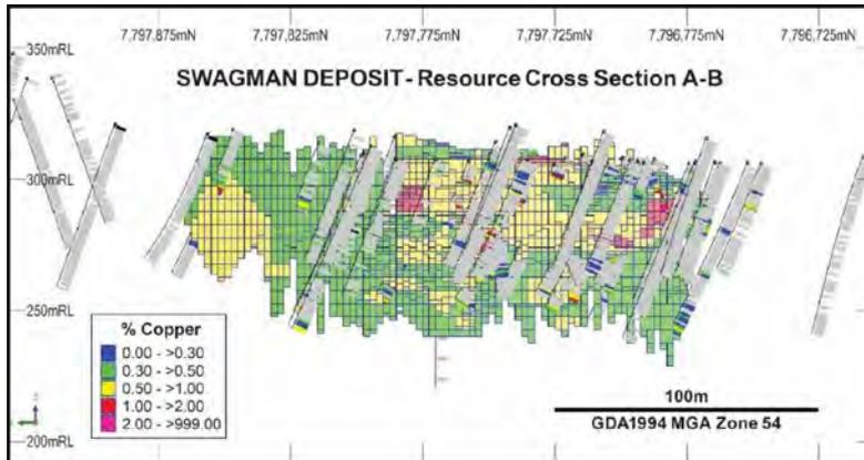
Figure B15: Cross section of the Swagman deposit showing drillholes and copper grade ranges of resource model blocks
